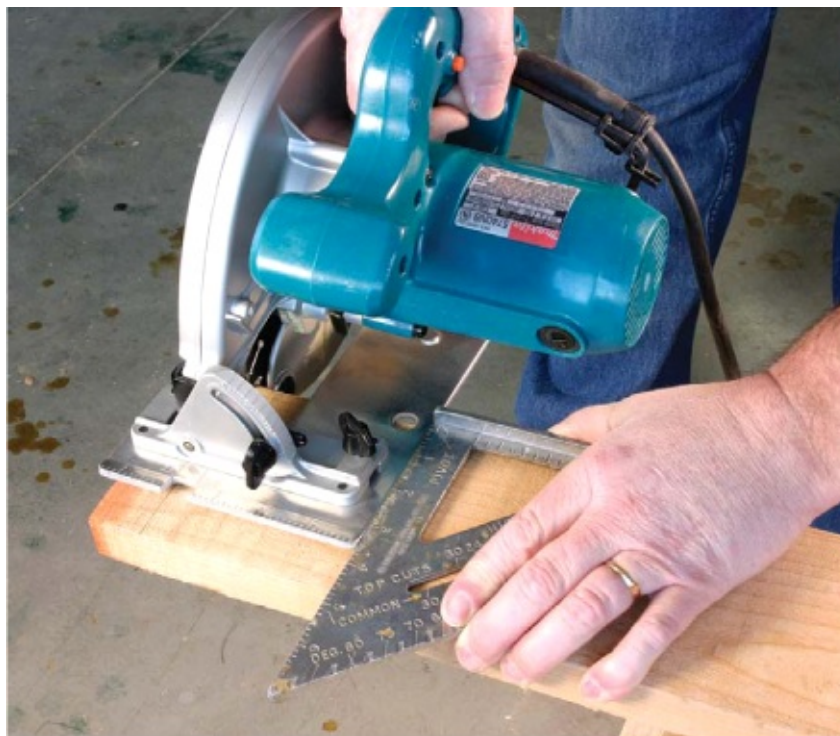
Aligning the blade with the cut line and using a speed square provides a temporary fence for a square or straight cut.
