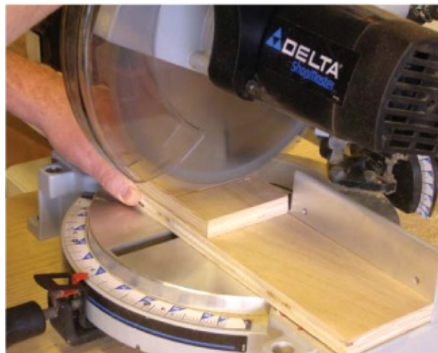
A miter saw makes short work of crosscutting the narrower piece. Put a piece of scrap beneath the
