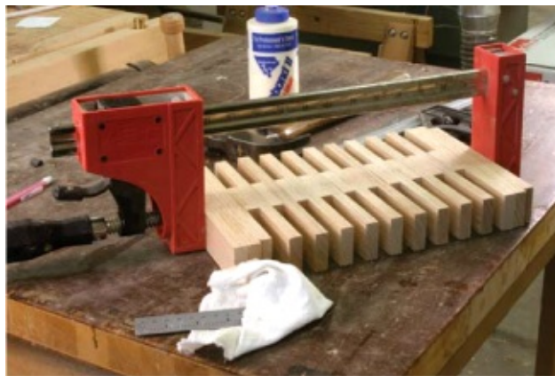
A cleaning rule. A damp rag over the end of a 6" rule is handy to get in between the pieces for glue cleanup.
