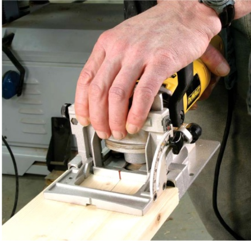
An alternate way to plunge: Squeeze the fence and tool handle together to make the cut.
