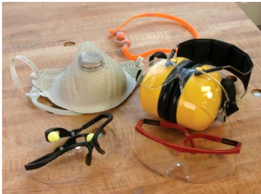
Safety gear — safety glasses, hearing protection and some type of dust mask — should always be used
