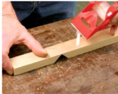
Tape as a hinge. Clear packing tape holds the ends of the joints together, and it lets you see what is happening as you assemble the joints.
