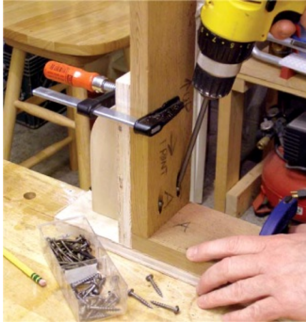
A shop-made right-angle clamping fixture keeps the drilled workpieces securely in place when driving the pocket screws
