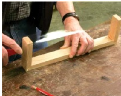
And as a clamp. Fold the ends up and use the tape to hold the parts in place while the glue dries.
