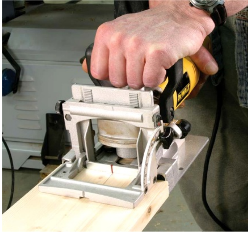
A textbook way of holding a biscuit joiner. Note that Bob's hip is braced against the rear of the tool. He'll shift his body forward during the plunge cut and use his arms to steady the tool.
