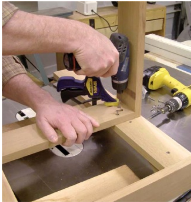
Attach the completed seat box to the leg sets with three countersunk 1¼ screws. Scrap wood under the leg set keeps everything level.
