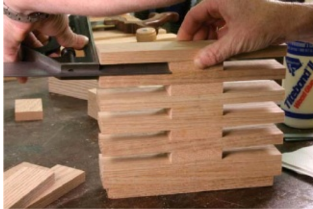
A fish ladder. Keep stacking until all your pieces are used, then cap with one of the “sandwiches.”
