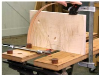
Fairing a curve. A thin strip of wood makes the perfect tool for designing a curve.
