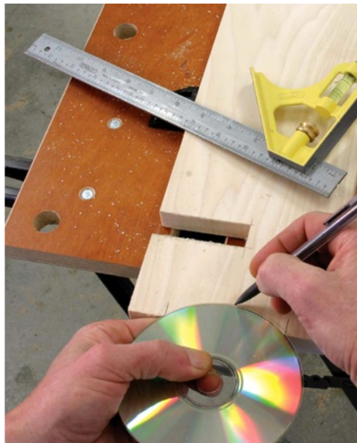
One simple joint is all it takes to build these shelves. The decorative cut is laid out by tracing the edge of a CD.
