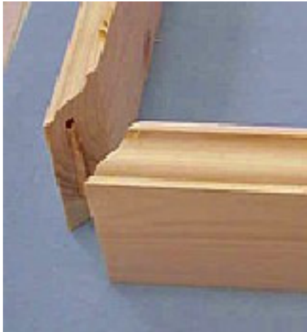
Miter joint with biscuits
