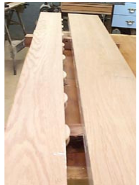
Biscuits used to reinforce part of a tabletop
