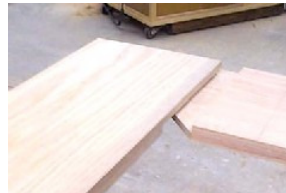
Mitered lap joint
