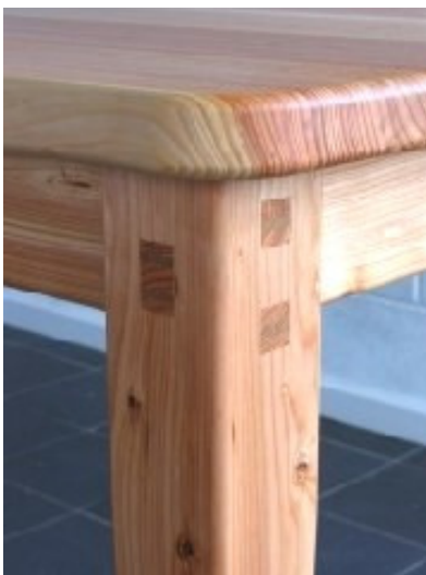
Figure 48: Method of attaching leg to rails of a table
