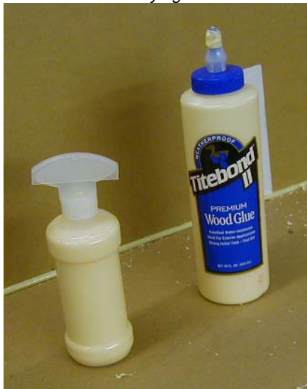
A special glue applicator for biscuit slots
