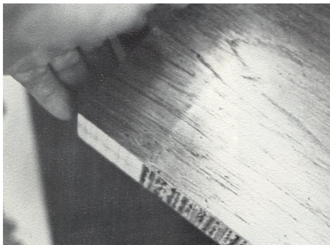
Figure 37: Junction of paper honeycomb and lumber band telegraphed through surface veneer
