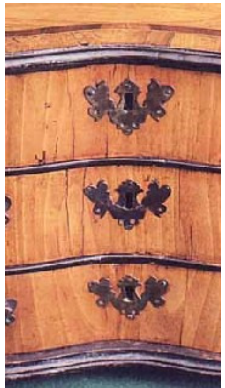
Figure 35: An example of veneer splitting over a wooden core
