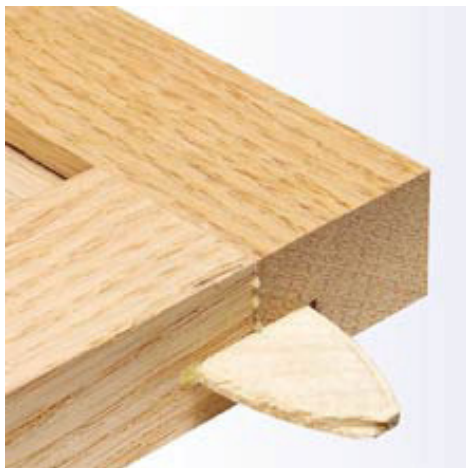
A biscuit used to reinforce a corner joint
