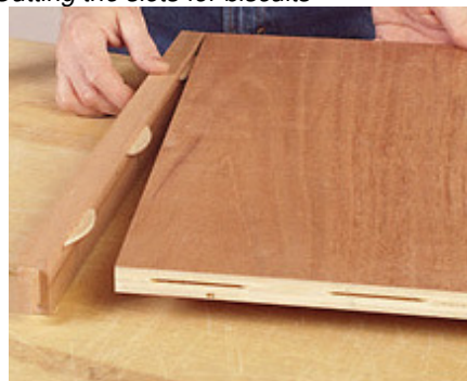
Dry assembly ensures proper alignment
