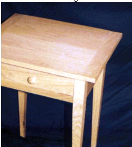
Figure 33: New lumber-banded panel used for a tabletop may rupture with aging.
