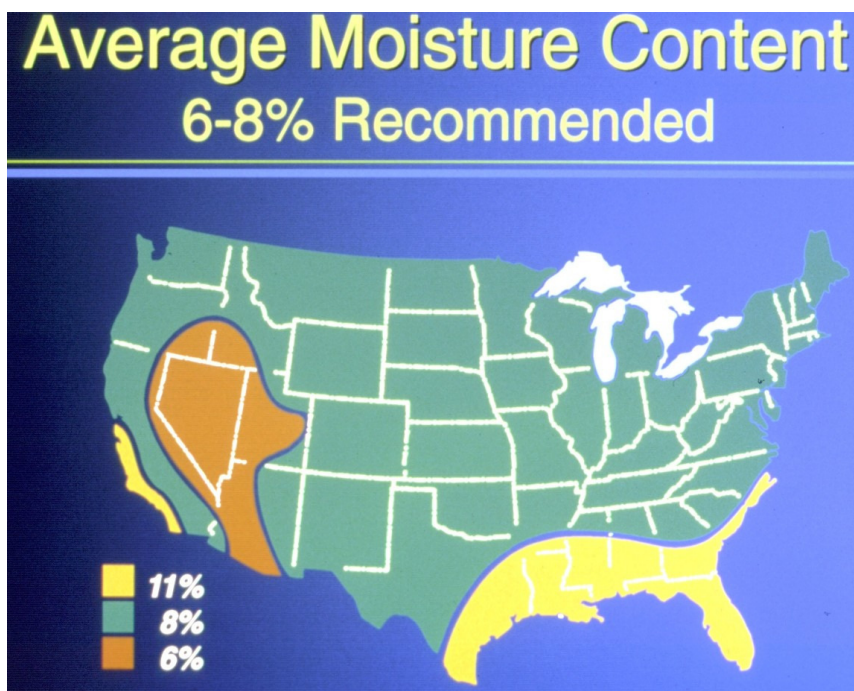
Figure 29: Recommended moisture content averages for interior-finishing woodwork for use in various parts of the United States
