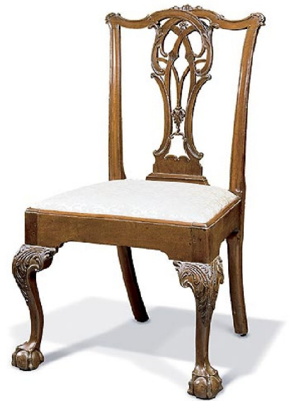
Figure 8: Chair with side rail flared at ends to increase glue joint strength.
