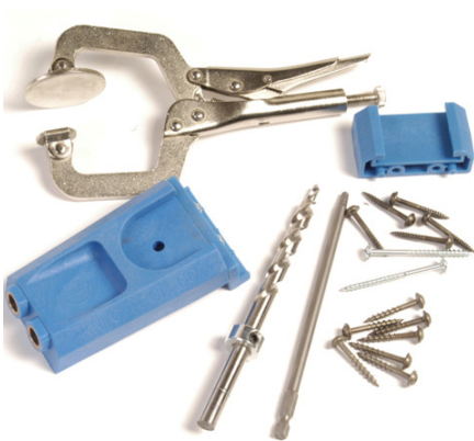
Tools used to drill a pocket hole
