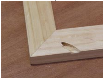
A pocket hole used to reinforce a mite joint
