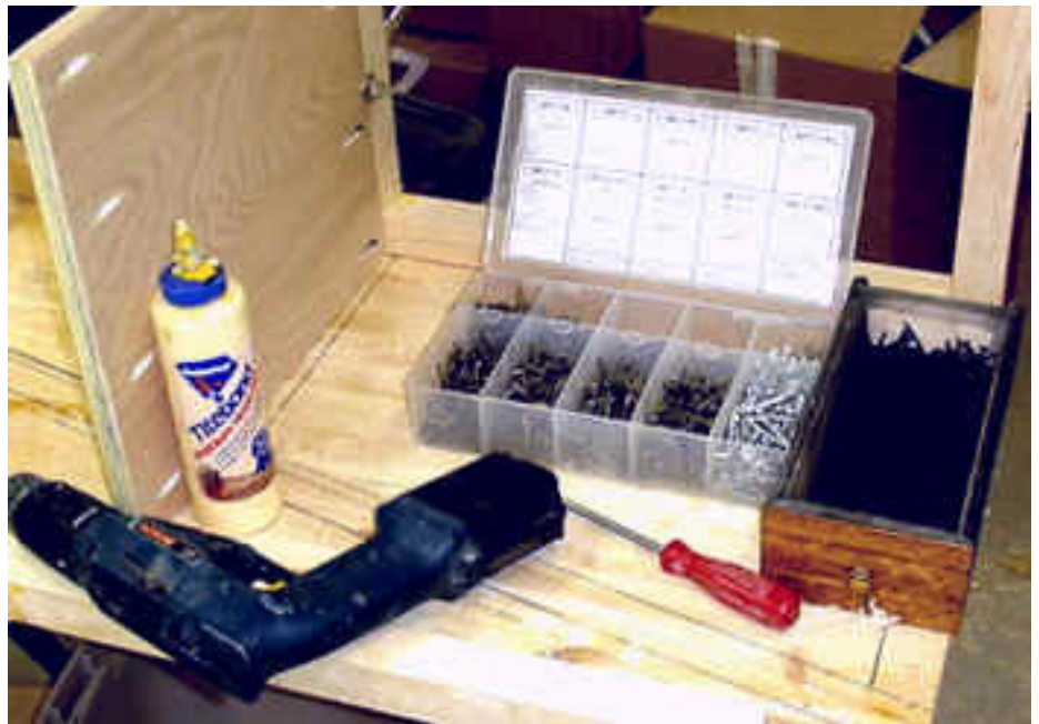
Preparing to assemble pocket hole joints with screws and Titebond II Premium Wood Glue
