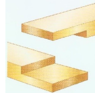
lap corner frame joint
