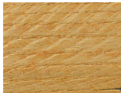
Figure 13: A dull, vibrating or out-of-line saw will give a poor glue joint, yielding lower strength, slower set, and lower wood failure.
