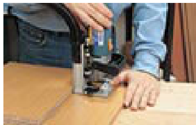
Cutting the slots for biscuits
