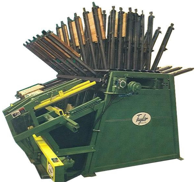
Figure 32: The above clamp carrier applies pressure evenly on stock for face gluing. Note the reinforcement blocks.
