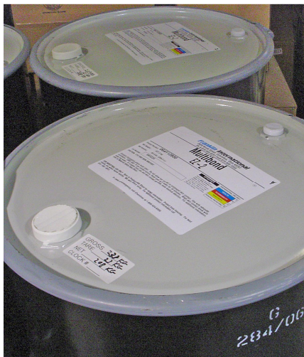
Figure 15a: Both 55-gallon and 30-gallon drums are provided with a 2" bung in the head so that a valve can be used.
