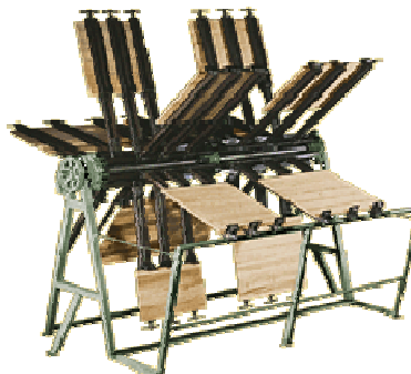
Figure 33: An example of a manual clamp carrier
