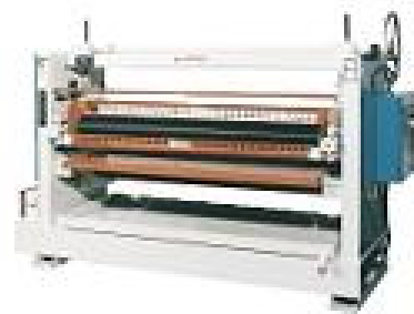
Figure 56c: A double roll spreader can spread both sides of either a core or veneer with one pass.
