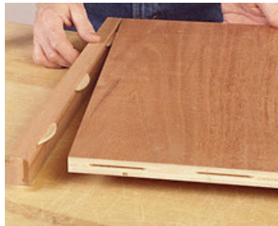
Dry assembly ensures proper alignment
