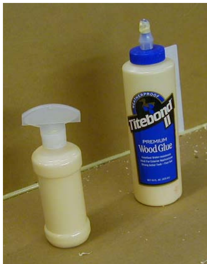
A special glue applicator for biscuit slots
