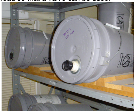
Figure 15b: The five-gallon pails have a built-in pour spout for easy dispensing of the glue.
