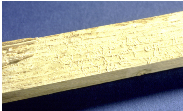
Figure 31: All illustration of a glue line showing the results of inadequate pressure.
