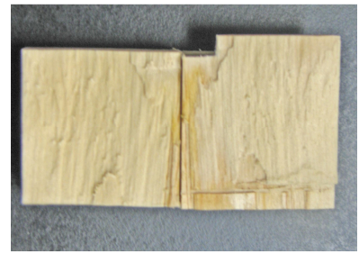
Figure 4: A good wood glue should yield high wood failure on hard maple when given the block shear test.
