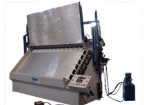
Figure 50: This radio frequency gluer is for doors and applies pressure in both directions. It will cure the adhesive in an assembly in as few seconds without the need for mechanical fasteners.
