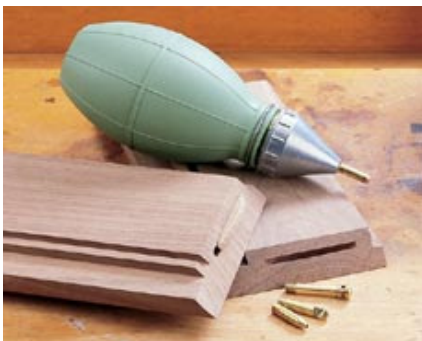
Figure 41: The brass tips, shown above, give better glue distribution and last longer than plastic tips. Some are designed for dowel holes, some for grooves.
