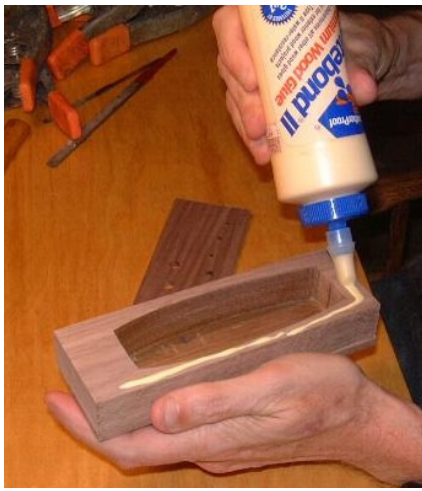
Applying glue using the bottle tip.
