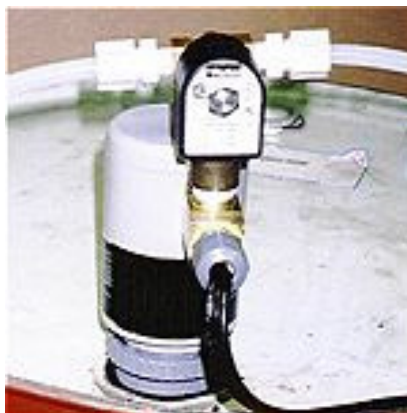
Figure 16: This pump can be installed in the 2" bung of a 55-gallon drum and used to pump adhesives throughout the plant. For water based adhesives, this should be stainless steel. For filling bottles a 1:1 pump is satisfactory, although for pumping any distance a 6:1 or 8:1 pump is required.
