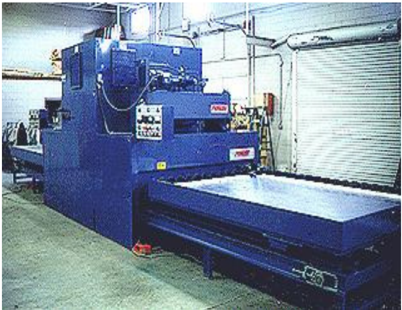
Figure 36a: A radio frequency gluer, with the appropriate adhesive, can decrease press time from more than 30 minutes to less than a minute. Figure 32B shows a hand-held radio frequency gluer.
