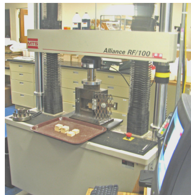
Figure 3: An testing machine equipped with a block shear attachment to run ASTM D-905
