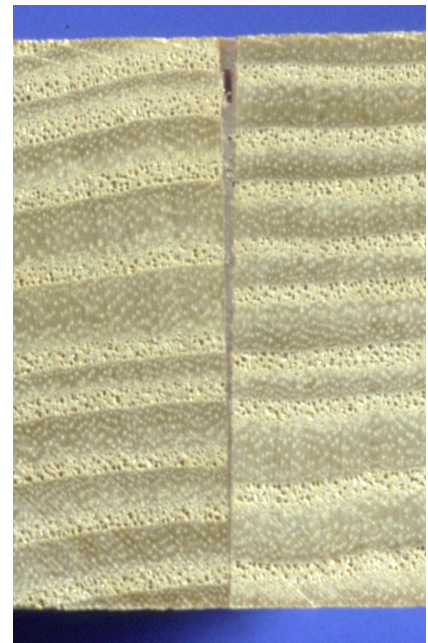
Figure 37: A thick glue line will produce a weak bond. This is a v-joint, which is the result of a poor fit or improper clamping. A thick glue line can also result from a long assembly time.
