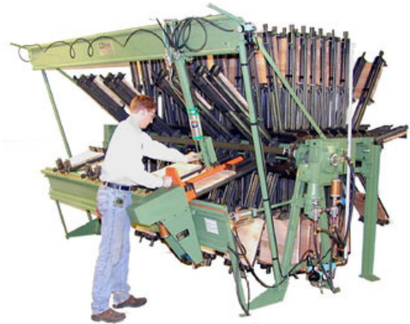
Figure 35: The addition of pneumatics or hydraulics to tighten the clamps is an improvement on the clamp carrier.
