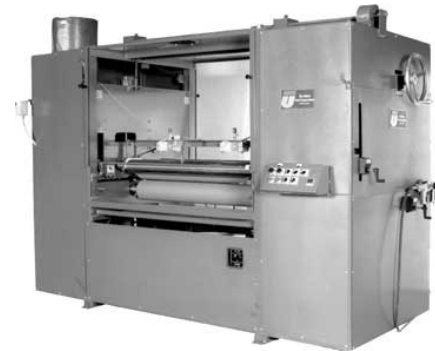
Figure 56a: An example of a hot melt roller coater
