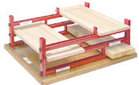
Figure 34: If production does not justify a clamp carrier, stacking clamps are useful.
