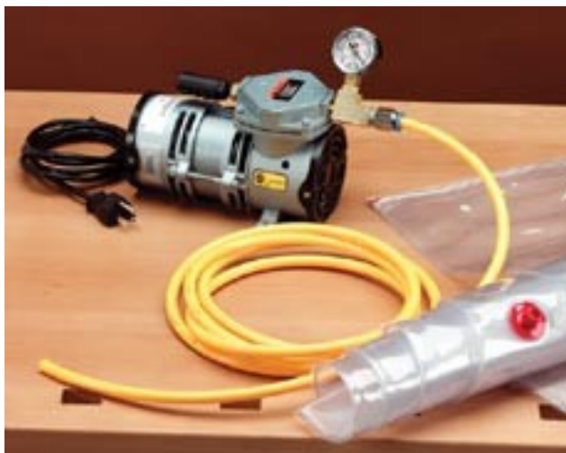
A small vacuum press with an electric pump
