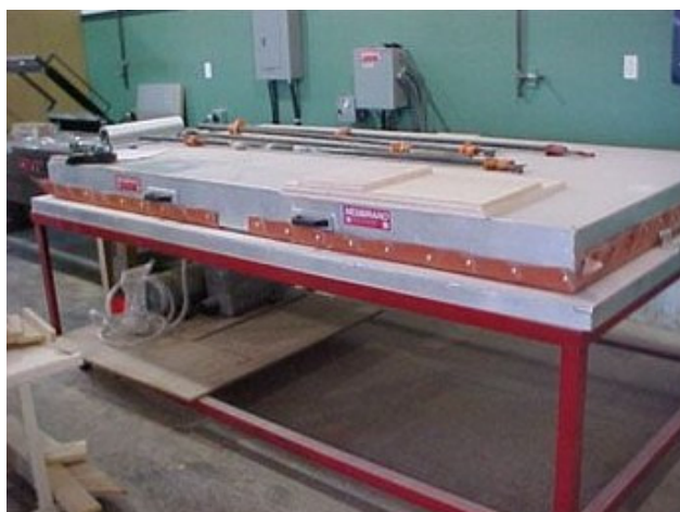
Figure 40a: A large vacuum press suited for plant use
