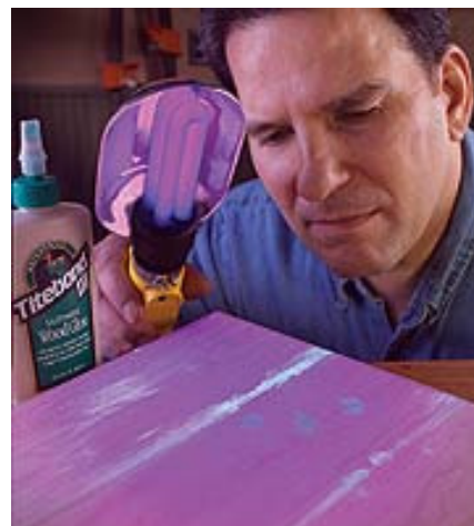
Figure 19: Use of a fluorescent dye in the glue will enable you to remove all of the squeeze-out.
