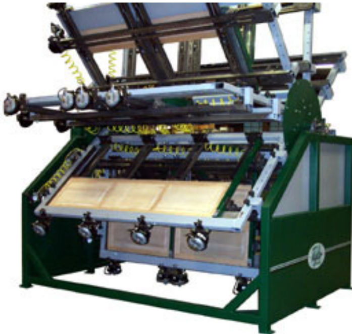
Figure 49: This clamp carrier applies side pressure in both directions during the cycle time.
