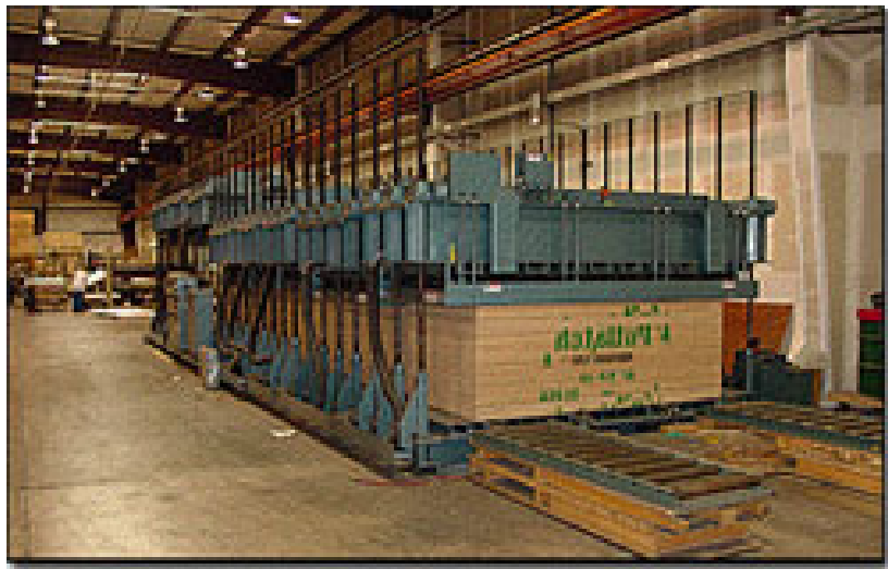
Figure 58 An example of a large cold press
