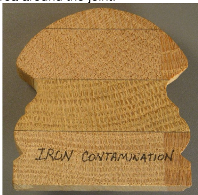
Figure 10: Note the dark discoloration on the oak from dissolved iron in the glue, which normally dries colorless.
