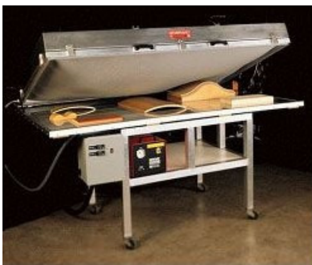
A vacuum press with a cover, as opposed to a bag
