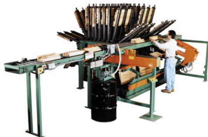
Clamp carrier and glue spreader
