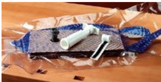
A small vacuum press with a hand pump
