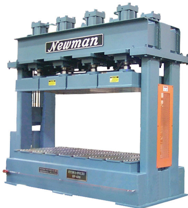
Figure 57: A large side loading cold press.
