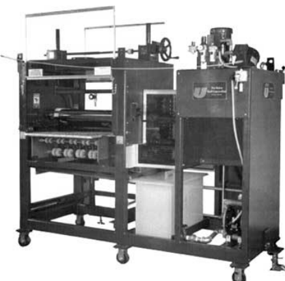
Figure 56a: Another example of a roller coater
