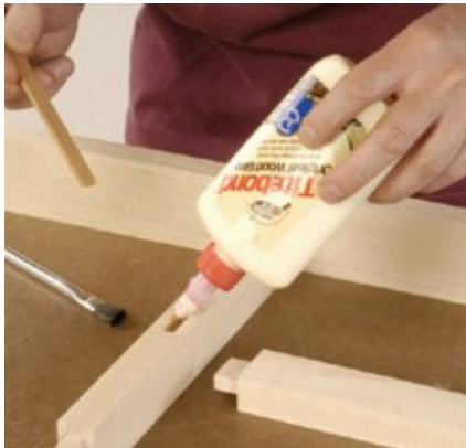
Applying glue with the aid of a stick and brush to smooth to an even coating.
