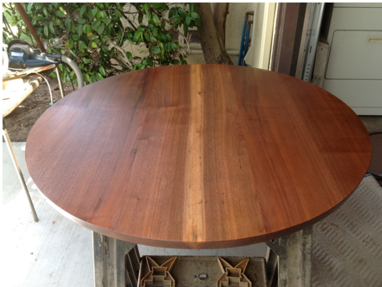
The effectiveness of oxalic-acid bleach is clear from this after picture.
